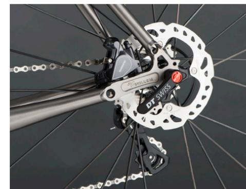
finish adorned with discreet branding, detailed in a mix of embossing, sandblasting and decals. The welding is clean, and there are some very neat touches, such as the internal routing of the gear cables on the side of the head-tube. The cast rear dropouts are also particularly gorgeous.
